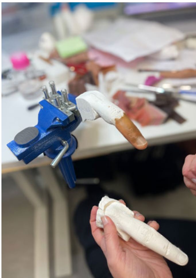
Above: Cosmetic silicone finger in the manufacturing process and the final devices for fitting.
